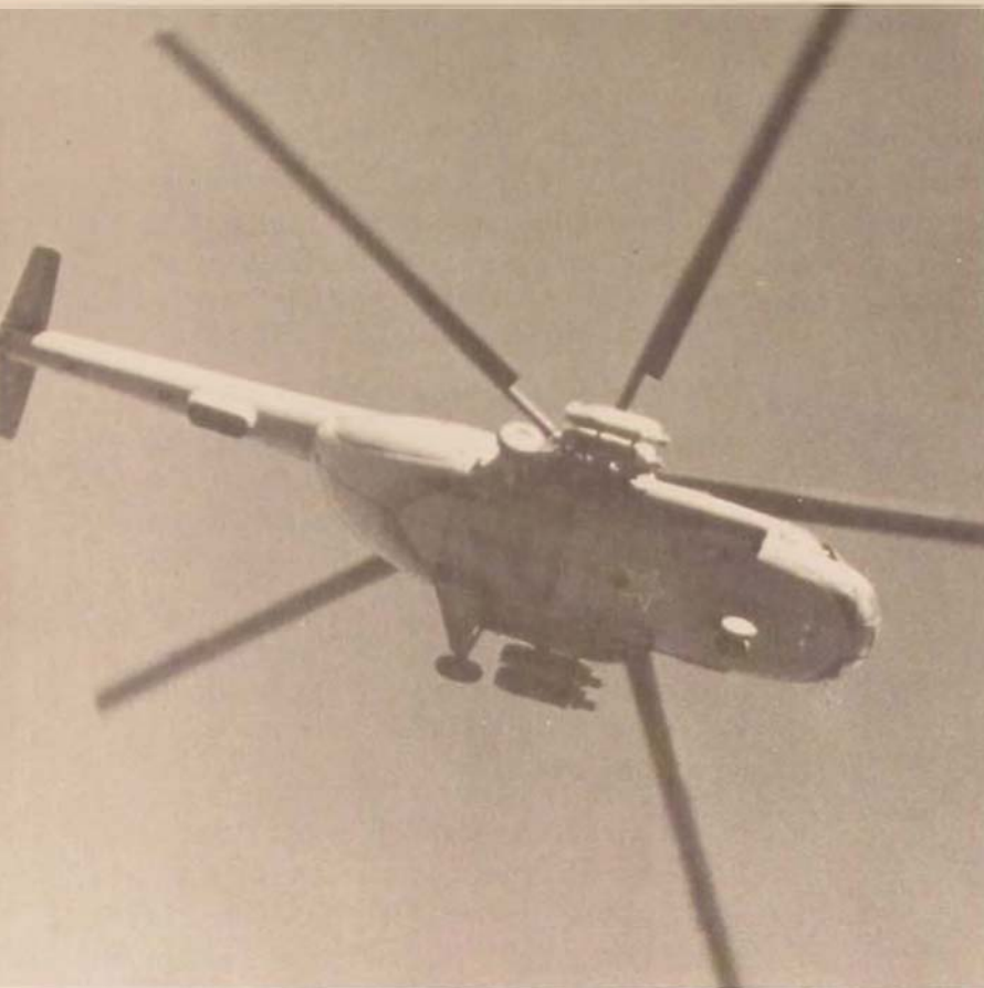
A Soviet Mi-8 Hip (left), equipped with external stores, can be fitted with an electrically operated rescue hoist above the left cabin door. Hips can be used as gunships, transports, or rescue helicopters. . . . Afghan freedom fighters stand triumphant over a downed Mi-4 Hound helicopter (below). The Mi-4 entered production in 1952 and is comparable to the Sikorsky H-19, which left the USAF inventory in the early sixties.
